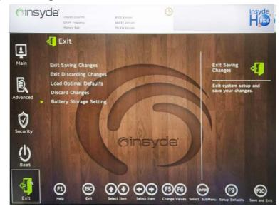
Click *Exit Saving Changes* (or press **F10**) to save all changes made and exit the BI-OS. Choosing *Exit Discarding Changes* will wipe out any changes you have made to the *Setup* and exit the BIOS. You can also choose to **Load Optimal Defaults** (or press **F9**) to return the *BIOS* to its original state, and erase any previous changes you have made in a previous session. Select **Discard Changes** to cancel any changes made in the current session.
