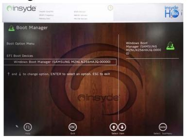
When you turn the computer on it will look for an operating system from the devices listed in this menu, and **in this priority order**. If it cannot find the operating system on that device, it will try to load it from the next device in the order specified in the **Boot Option Menu**.
