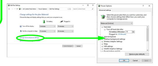
Each *Windows* **power plan** will also adjust the processor performance of your machine in order to save power. This is worth bearing in mind if you are experiencing any reduced performance (especially under DC/battery power).
