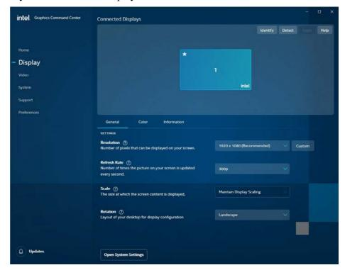
Use the Display menu to adjust the display's Resolution, Refresh Rate, Scale, and Rotation, and to access the Display control panel in System Settings.
