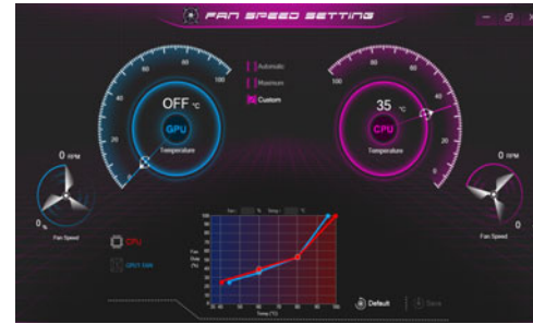
Figure 8 - Fan Speed Control
