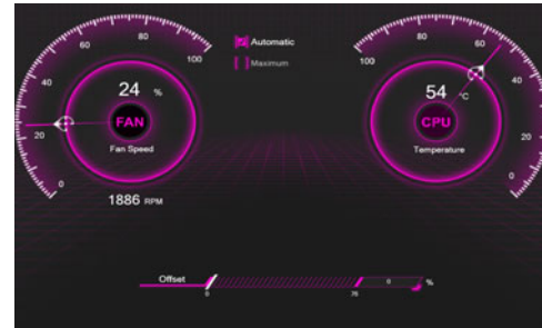
Figure 10 - Fan Speed Control
