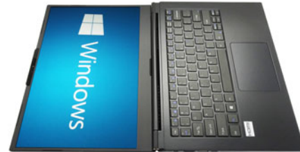
Figure 4 - LCD Panel Open to 180 degrees with Screen Rotated
