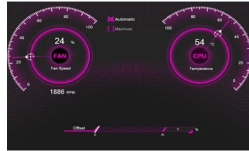
Figure 14 - Fan Speed Control
