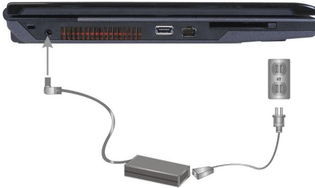
3. Plug the connector of the AC adapter to the DC-IN port found at the left side of the computer.
