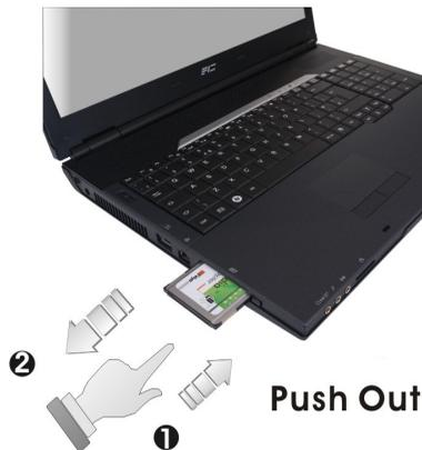
**NOTE** *The power consumption of ExpressCard/54 is about 2.1W, while the consumption of ExpressCard/34 is about 1.3W. To save energy, press the button to disconnect the card when it is not in use.*
