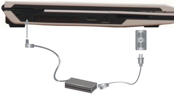
3. Plug the connector of the AC adapter to the DC-IN port found at the left side of the computer.
