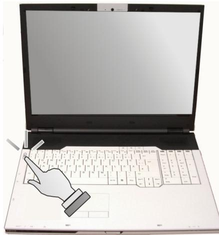
After a few seconds, the computer's display will turn on and your computer will begin to execute the Power On Self Test or POST to check if all system components are running properly. Any error found during the test will be displayed on the screen and may generate short beep sound as well.
