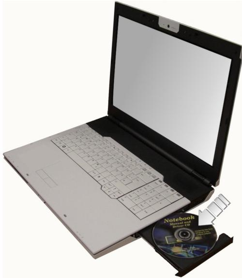
3. To remove the disc, press on the center spindle and pull up the disc from the side until the disc snaps out of the spindle lock.
