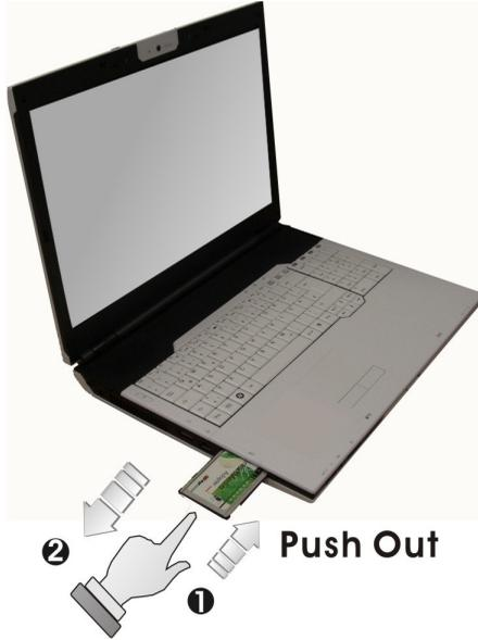
**⚠** *The power consumption of ExpressCard/54 is about 2.1W, while the consumption of ExpressCard/34 is about 1.3W. To save energy, press the button to disconnect the card when it is not in use.*
