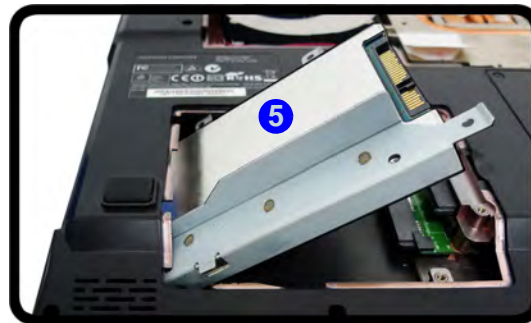
Figure 6 - 9 Secondary HDD Assembly Removal
