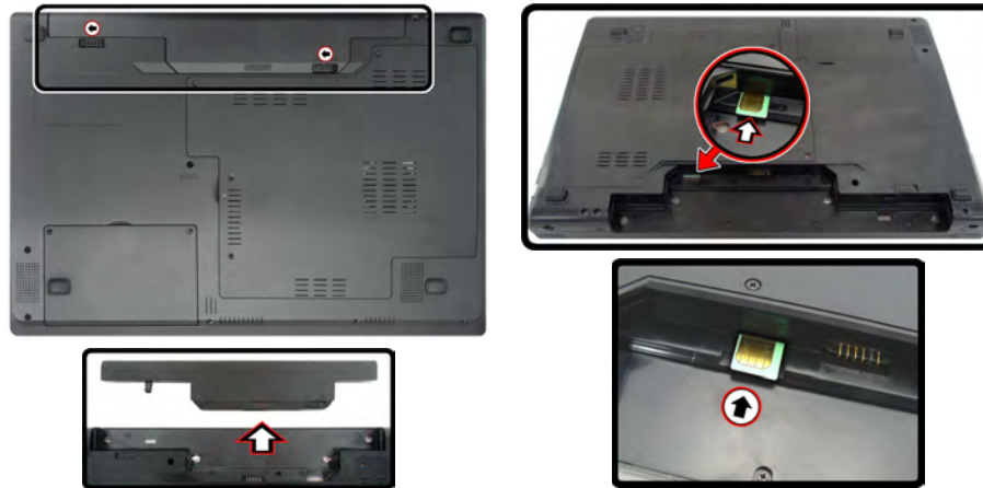
Figure 1 - 9 - Battery Removal & USIM Card Insertion
