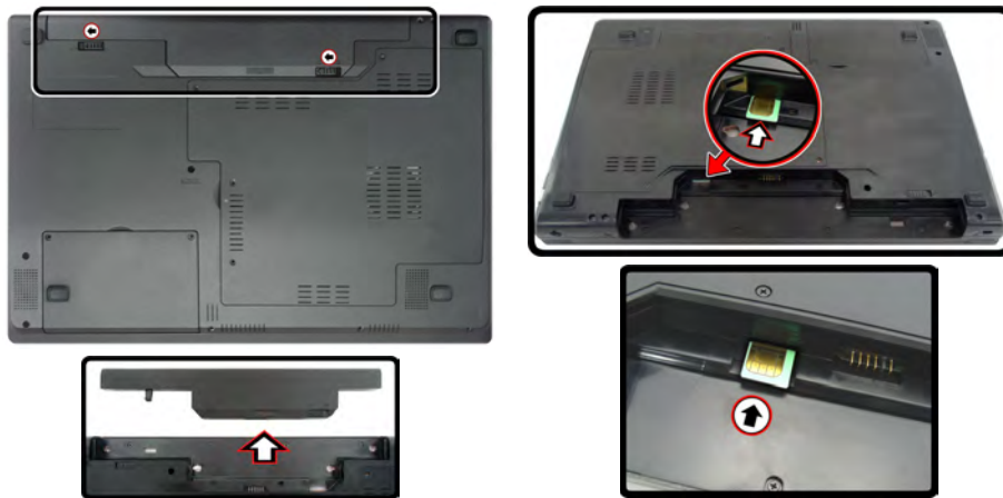
Figure 1 - 9 - Battery Removal & USIM Card Insertion
