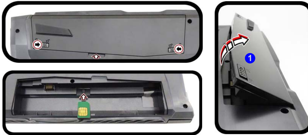
Figure 26 - Remove the battery and Insert the USIM Card
