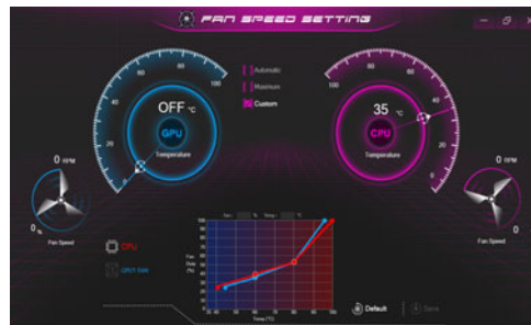
Figure 9 - Fan Speed Control
