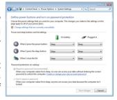
Sleep is the same as Suspend-to-RAM (STR). This function stores your current data and status in RAM while many components are turned OFF. Because RAM is volatile, it requires power to keep (refresh) the data. Click the Start button and the arrowhead next to the lock icon to see this option. You can also use the keyboard shortcut [Fn F1] to activate this mode. Recover by pressing any keyboard key except [Fn]. (NOTE: The power indicator will blink in this mode.)
