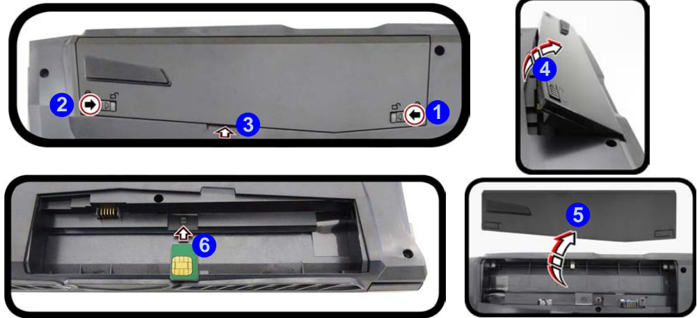
Figure 1 - 15 Battery Removal & USIM Card Insertion
