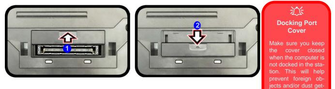
Figure 1 - 12 - Opening and Closing the Docking Port
