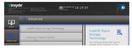
Figure 6 - 2 Intel(R) Rapid Storage Technology (Note this item only appears after you have restarted and accessed the BIOS again after having set **SATA Mode** to **RAID**)
