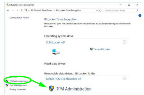
Figure 6 - 36 BitLocker Drive Encryption (TPM Administration) 4. The TPM Management window allows you to configure the TPM within *Windows*. As TPM is usually administered within large enterprises and organizations, your system administrator will need to assist you in managing the information here.
