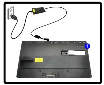
Figure E - 8 - Docking Station with AC/DC Adapter Plugged
