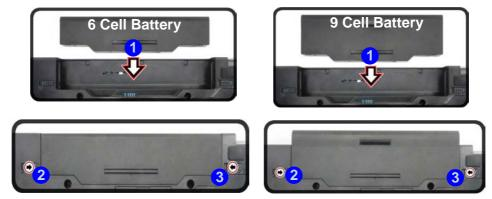
Figure 1 - 11 - Battery Insertion
