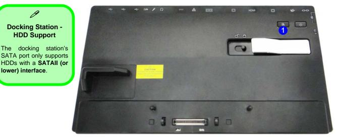
Figure E - 13 - Front View (HDD Backup Hotkey)
