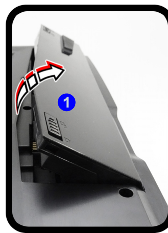
Figure 27 - Remove the battery and Insert the USIM Card
