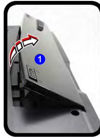
Figure 28 - Remove the battery and Insert the USIM Card
