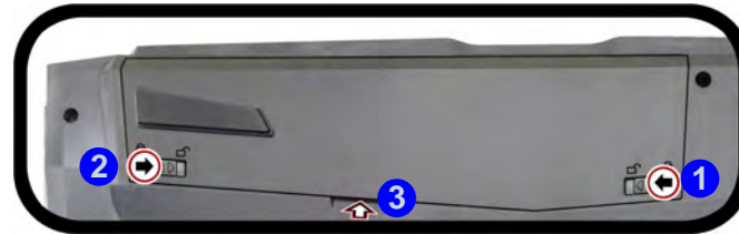
Figure 6 - 47 Battery Removal & USIM Card Insertion
