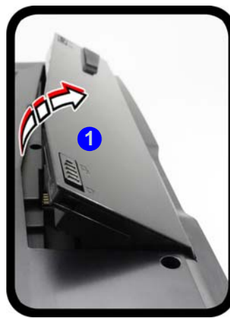
Figure 33 - Remove the battery and Insert the USIM Card
