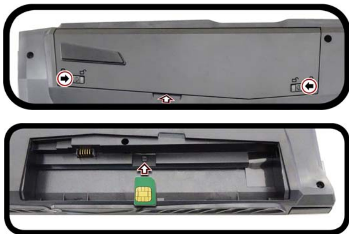
Figure 33 - Remove the battery and Insert the USIM Card
