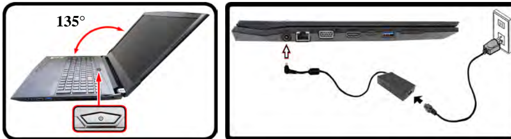
Figure 1 - 1 - AC/DC Adapter In / Opening the Lid/LCD
