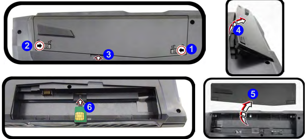
Figure 1 - 19 Battery Removal & USIM Card Insertion
