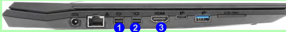
Figure 1 - 18 - Left Side View (Mini Display Ports & HDMI Port Highlighted) - Single Model Pictured
