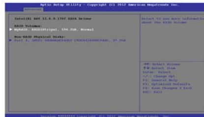
Figure 4 Informations RAID (Advanced > Intel(R) Rapid Storage Technology)
