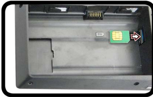
Figure 35 - Remove the battery and Insert the USIM Card
