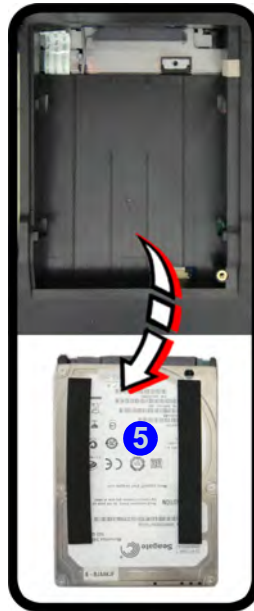
Figure 6 - 6 Primary Hard Disk Insulation Plate Removal
