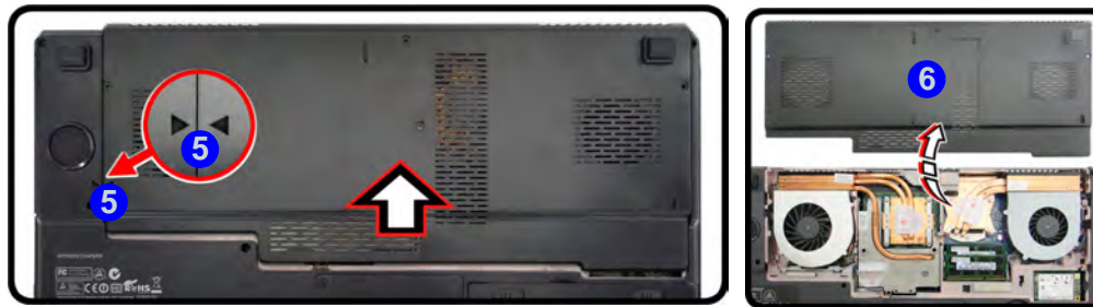
Figure 6 - 26 Component Cover Move & Removal (Model E)
