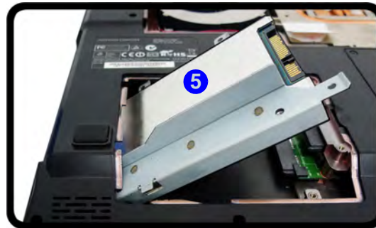
Figure 6 - 9 Secondary HDD Assembly Removal (Model C)
