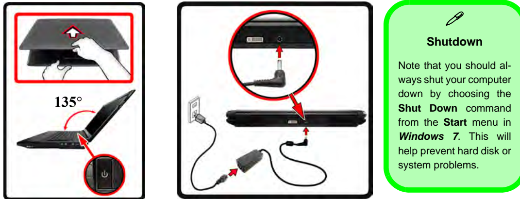
Figure 1 - 1 - Computer with AC/DC Adapter Plugged-In/Opening the Lid/LCD
