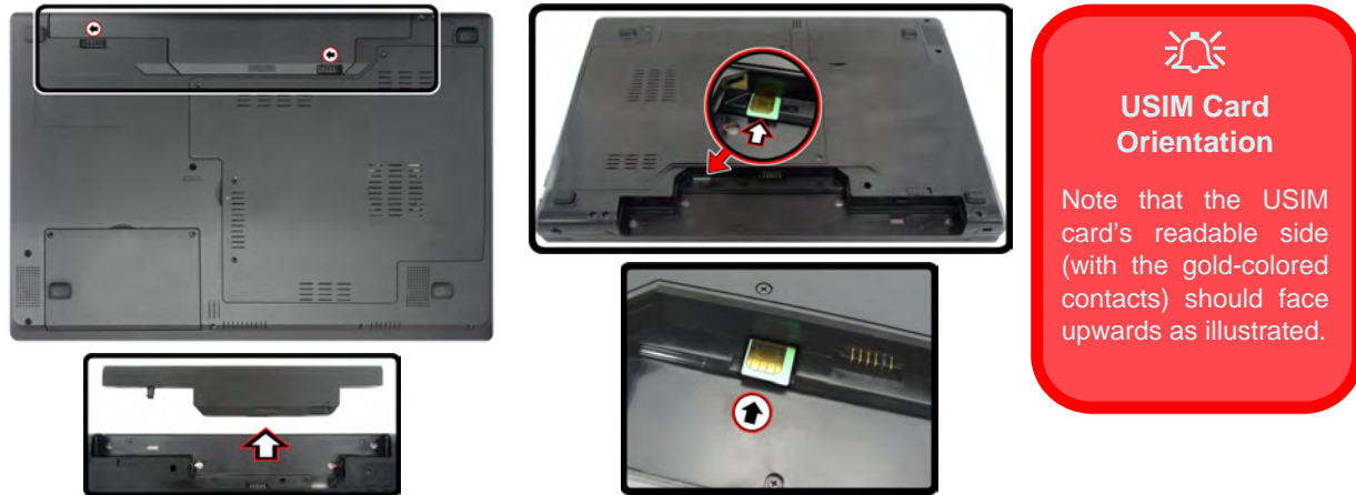
Figure 1 - 9 - Battery Removal & USIM Card Insertion
