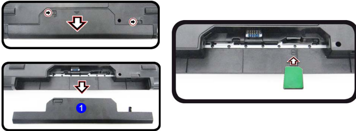
Figure 14 - Remove the battery and Insert the USIM Card
