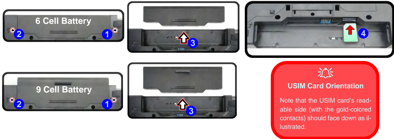
Figure 1 - 10 - Battery Removal & USIM Card Insertion
