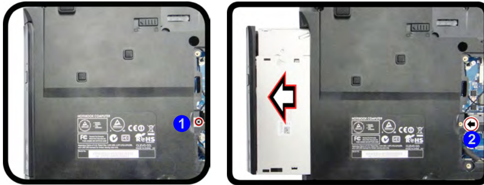
Figure 6 - 3 Removing the DVD Device
