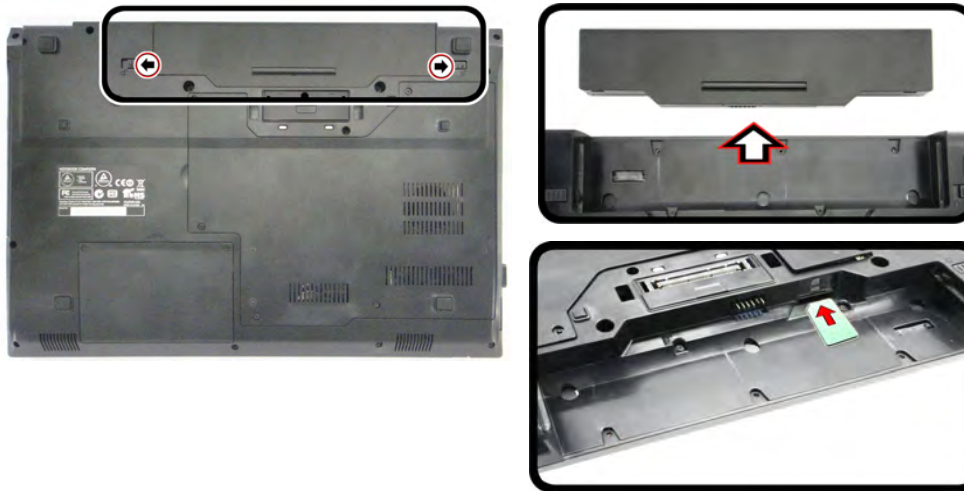
Figure 1 - 9 - Battery Removal & USIM Card Insertion
