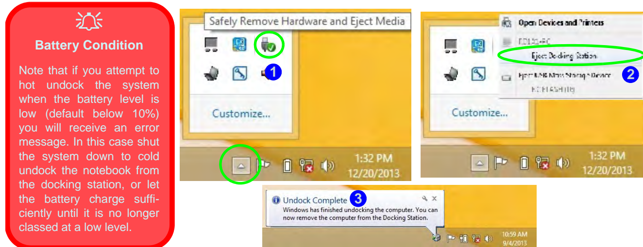
Figure E - 11 - Using the Windows System to Hot Undock the Computer
