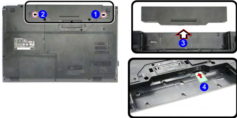
Figure 7 - 55 Battery Removal & USIM Card Insertion
