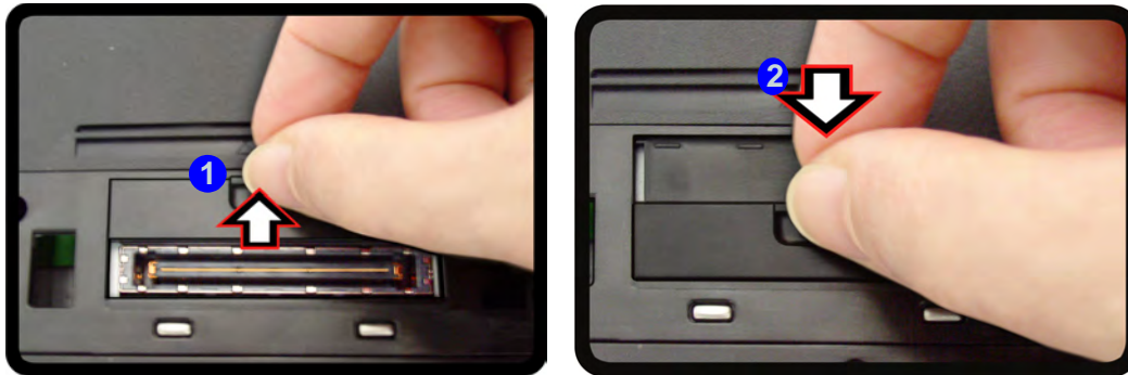
Figure 1 - 10 - Opening and Closing the Docking Port
