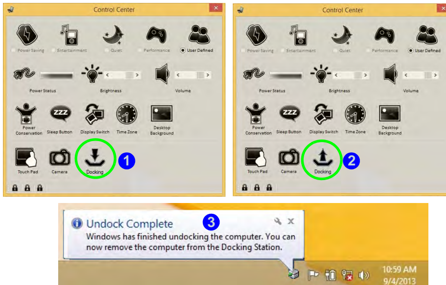
Figure E - 12 - Using the Control Center to Hot Undock the Computer
