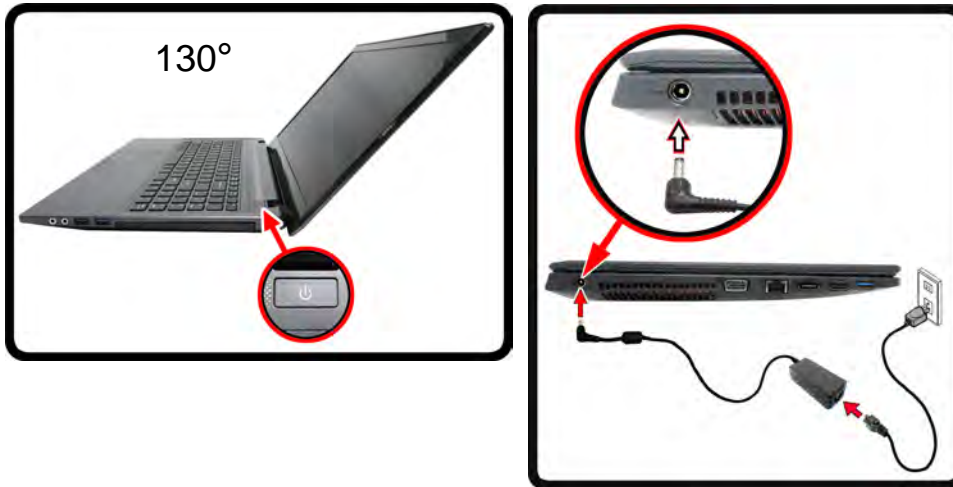
Figure 1 - 1 - Opening the Lid/LCD & Computer with AC/DC Adapter Plugged-In
