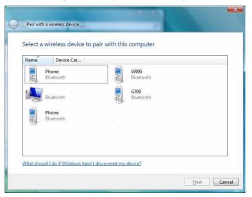
On first connection the computer will provide you with a pairing code to be entered onto the device. Enter the code into your Bluetooth enabled device and follow any on-screen instructions to complete the pairing.
