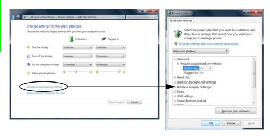
Each *Windows* **power plan** will also adjust the processor performance of your machine in order to save power. This is worth bearing in mind if you are experiencing any reduced performance (especially under DC/battery power).
