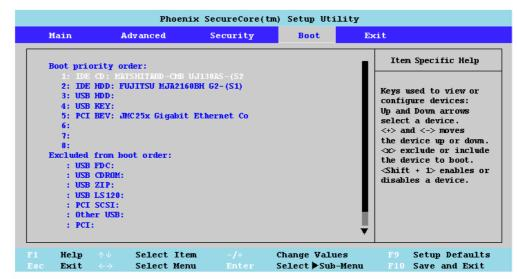
When you turn the computer on it will look for an operating system (e.g. *Windows Vista*) from the devices listed in this menu, and **in this priority order**. If it cannot find the operating system on that device, it will try to load it from the next device in the order specified in the **Boot priority order**. Item specific help on the right is available to help you move devices up and down the order.
