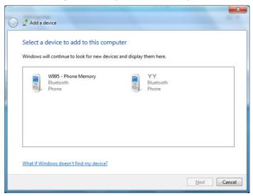
On first connection the computer will provide you with a pairing code to be entered onto the device. 4. Enter the code into your Bluetooth enabled device and follow any on-screen instructions to complete the pairing.
