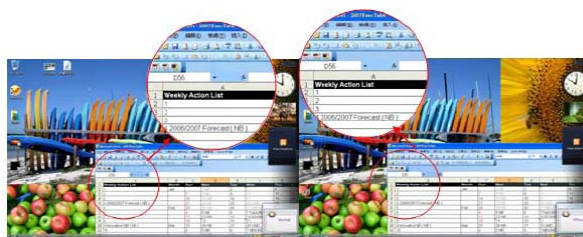
Figure 06: Comparing to Normal mode (circle right), Office mode (circle left) provides sharper edges on letters for better readability
