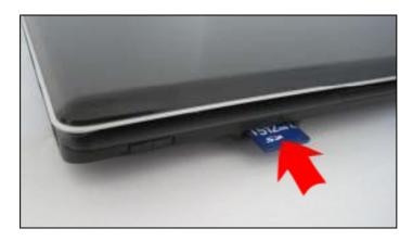
Hold the SD/MMC/MS card with its orientation symbol pointing into the slot and the topside of the card facing up.
