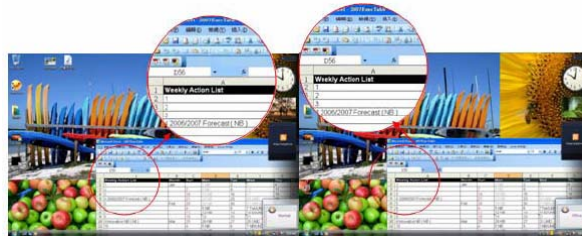
Figure 07: Comparing to Normal mode (circle right), Office mode (circle left) provides sharper edges on letters for better readability
