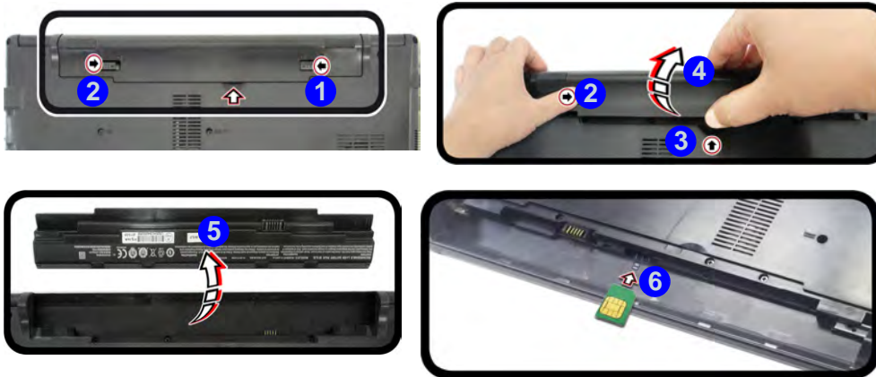
Figure 6 - 13 Battery Removal & USIM Card Insertion
