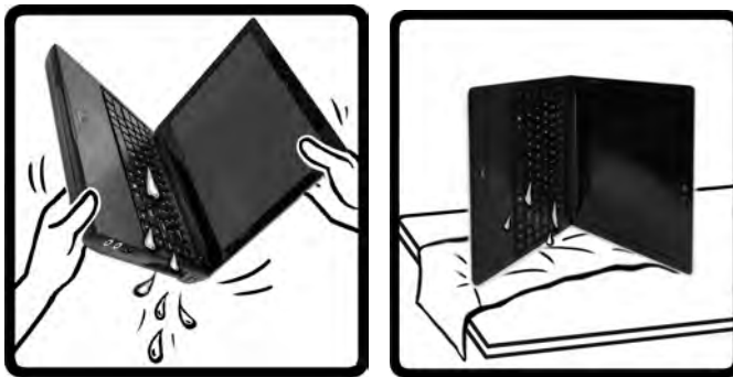
Figure 7 - Drain any Liquid to the Right Side and Rest the Computer on the Right Side to Dry
