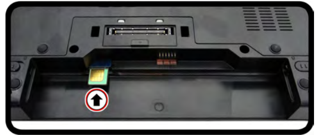
Figure 9 - Insert the USIM Card
