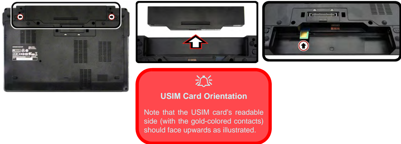
Figure 1 - 8 - Battery Removal & USIM Card Insertion
