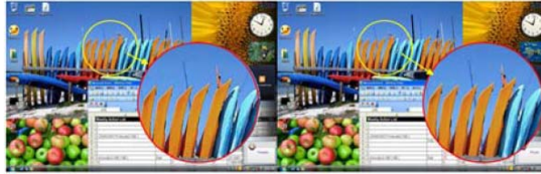
Figure 07: Photo mode (circle left) provides higher details on objects, While Movie mode (circle right) provides lower.
